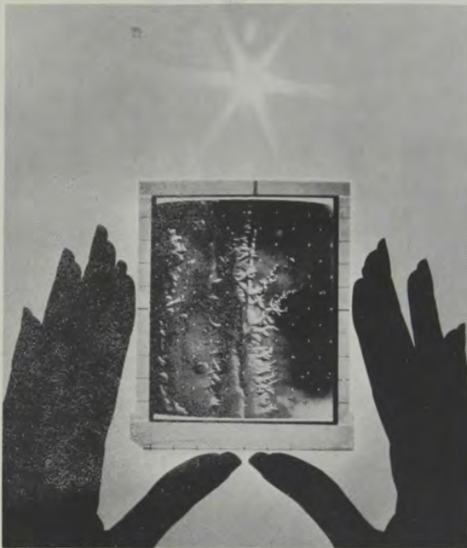
A Mariner photo is sent back in a radio stream of 580,000 signals coded for light-to-dark intensity. UNIVAC computer 1230 MTC takes those signals and enhances them subtly to make darks darker and lights lighter. The resulting contrast brings out obscure terrain features.
