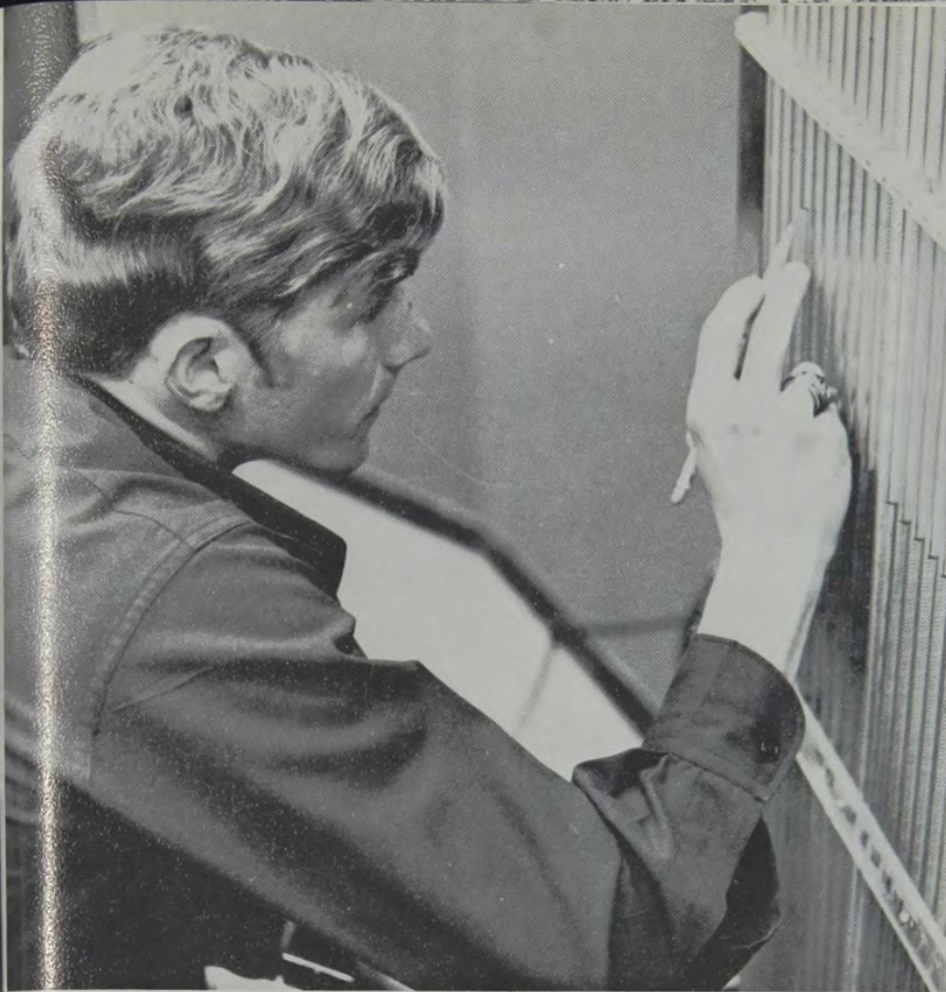
Cadet Dick Collins measures effects of a wind tunnel through the use of this manometer.
